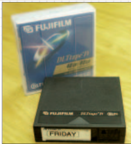
Backup tapes should be made daily and stored off-site separate of the database server.
