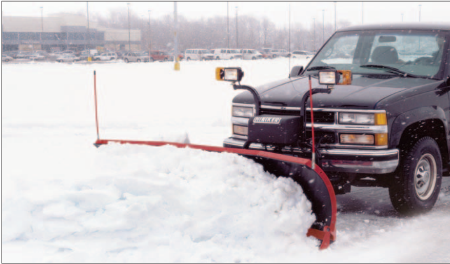
Identifying where a plow will be used, such as in a parking lot or on a residential street, is the first step in selecting the most appropriate model. The choice of a front-mounted, belly, or wing plow depends on its application within your fleet.
